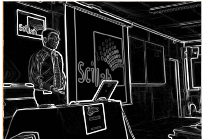
Figure 9. The edges as revealed by the Sobel filter.
