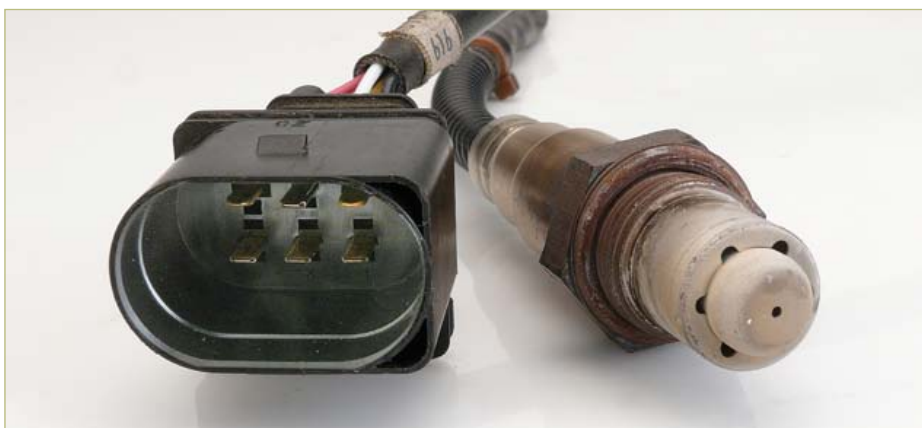
Figure 8. The lambda probe is supplied with a cable which includes a factory calibrated preset resistor.
